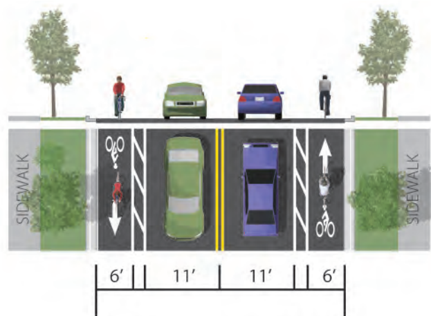
The proposed cross section for Main Street will include buffered bike lanes, two total travel lanes, park strip, and sidewalk
