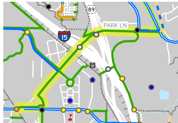
Context map of the Park Lane overpass and interchange area improvements, and the extents of the project highlighted in yellow (D&RGW Rail Trail to Main St). Blue lines represent proposed bike lanes, dashed bright green sidewalks, green shared-use paths, orange bicycle boulevards, and tan shared lanes. All dashed gray lines are existing facilities.
