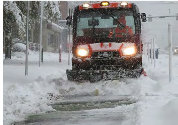
A small tractor with a narrow plow attached clears a separated bike lane during a winter snow storm in Salt Lake City (Photo: SLC Public Works)
