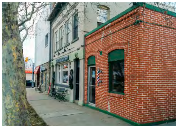
Some elements of pedestrian overlay districts are found on Farmington's Main and State Streets downtown, like zero-setback buildings, shade trees, and ground floor commercial uses
