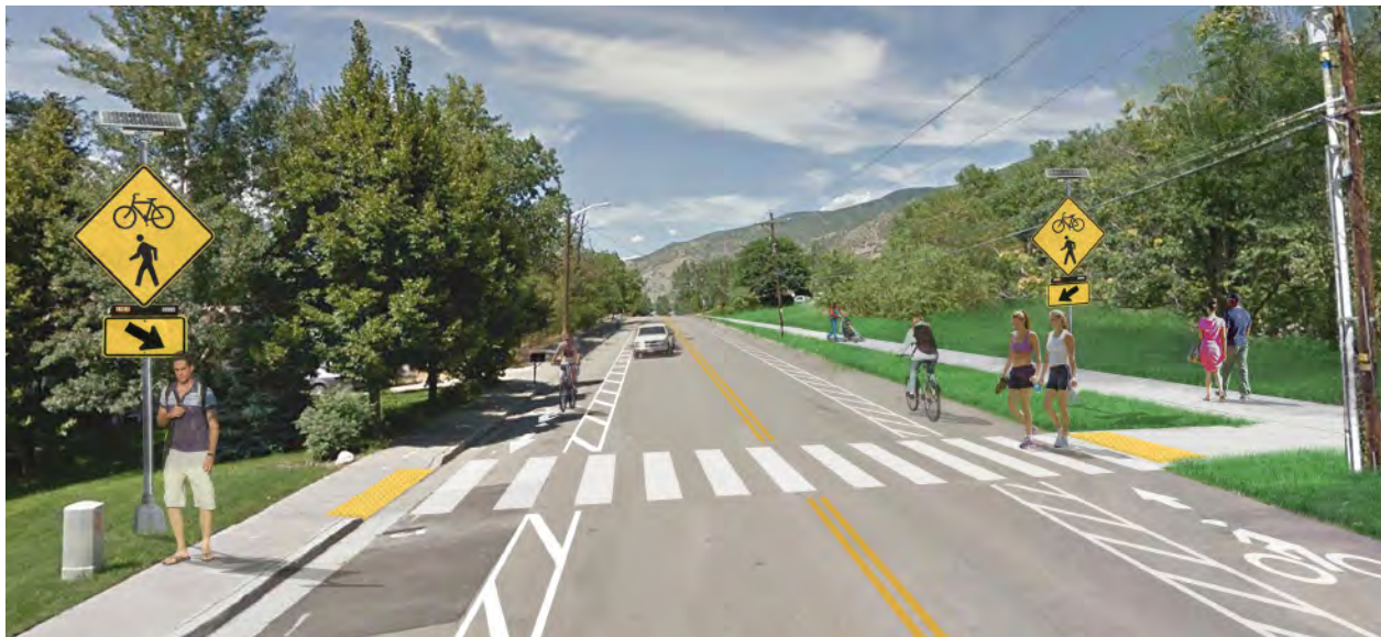
A rendering of what 200 East would look like after adding sidewalks and buffered bike lanes
